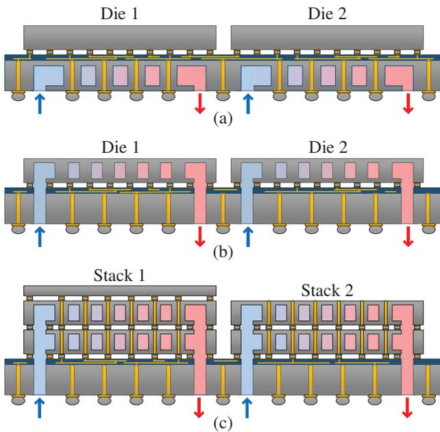
Fig. 2. Microfluidic cooling integrated in (a) the interposer, (b) the backside of the die, and (c) the backside of multiple dice in a 3D stack
