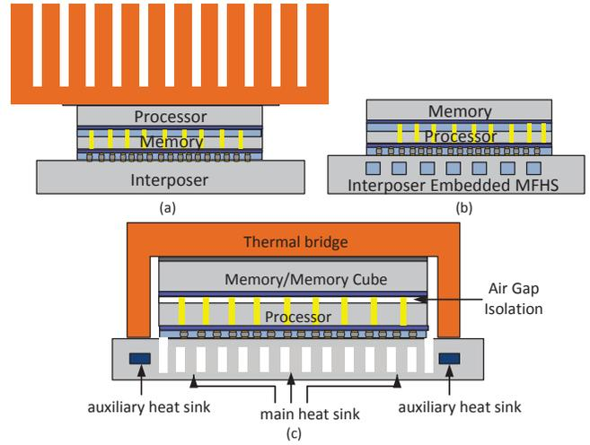
Fig. 13. (a)3D stack with air cooled heat sink (b)3D stack with interposer microfluidic cooling (c)Proposed stack with separate microfluidic cooling and thermal bridge
