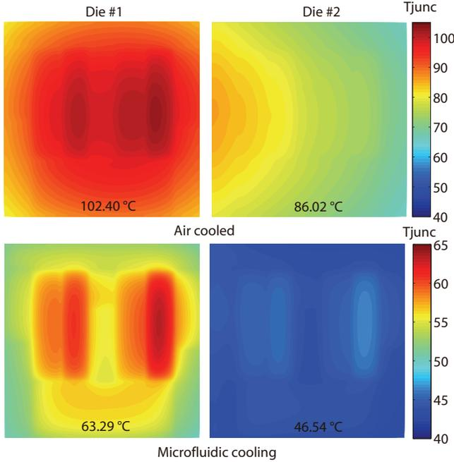
Fig. 11. Simulated temperature maps of the dice with microfluidic cooling and air cooling
