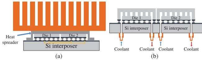
Fig. 10. Silicon interposer based 2.5D stacks using (a) conventional air cooled heat sink and (b) embedded die-specific microfluidic heat sink
