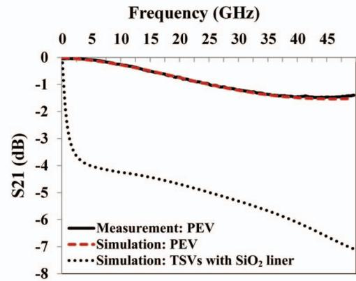
Fig. 6. Polymer-embedded via (PEV) measurement.
