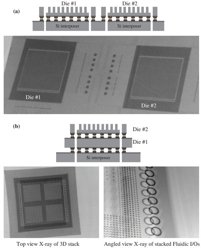
Fig. 9. Diagrams and X-ray images of (a) two silicon dice with microfluidic I/Os and embedded micropin-fin heat sink (2.5D) and (b) two silicon dice with microfluidic I/Os and embedded micropin-fin heat sink stacked on a silicon interposer (3D); top view X-ray image, and angled view of fluidic I/Os.
