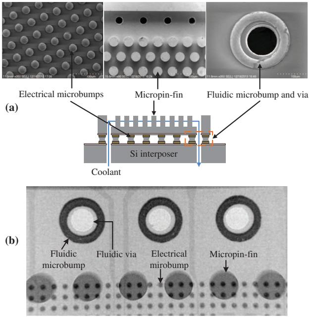
Fig. 7. a) SEM images of electrical microbumps, fluidic microbumps and vias, and micropin-fin heat sink on a silicon die; (b) X-ray images of the flip-chip bonded electrical microbumps, fluidic microbumps, and micropin-fins
