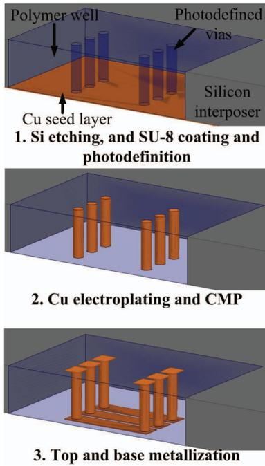
Fig. 4. Fabrication process for polymer-embedded vias.
