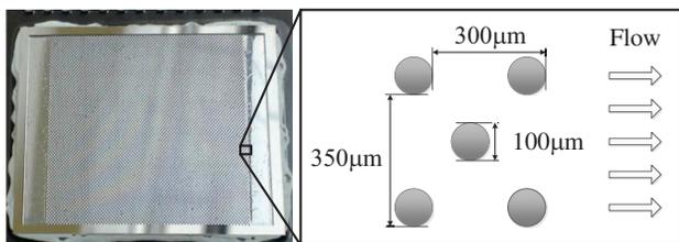
Fig. 15. Micropin-fin dimensions
