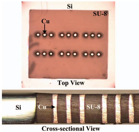
Fig. 5. Fabricated polymer-embedded vias.
