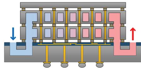
Fig. 3. Fluid can be routed through an interposer and delivered to monolithically integrated microfluidic heat sinks integrated into the backsides of dice.
