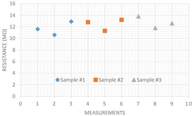
Fig. 8. Resistance of electrical microbumps measured on three bonded samples
