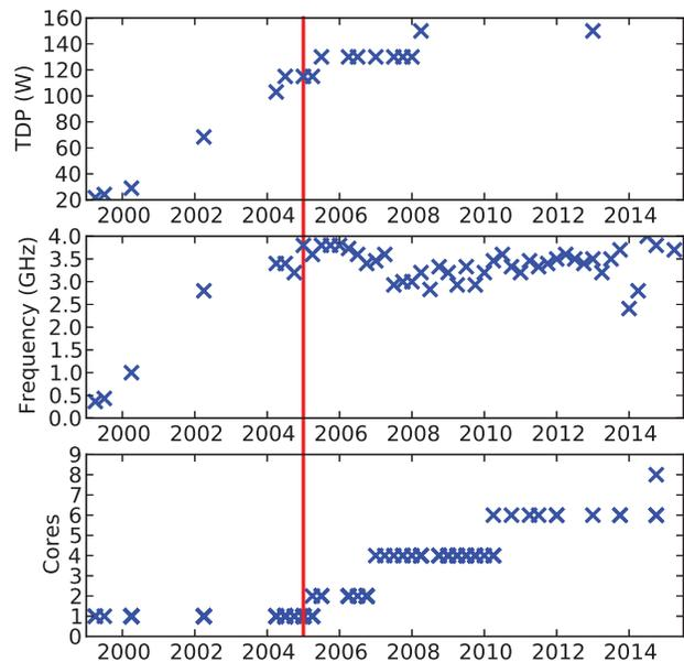
Fig. 1. Maximum thermal design power (TDP), clock frequency, and number of cores for Intel desktop CPUs
