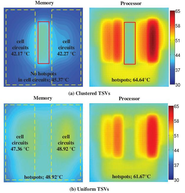
Fig. 14. Thermal maps of clustered TSVs and uniform TSVs (a) TSVs are clustered in the solid-line box (b) The same number of TSVs are uniformly distributed
